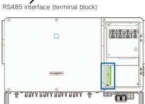
**i** RS485-1 terminal block interface and RJ45 interface serve as the same function with wiring manner different.
