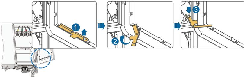
\*Close the wiring compartment in reverse order after completing wiring operations.
