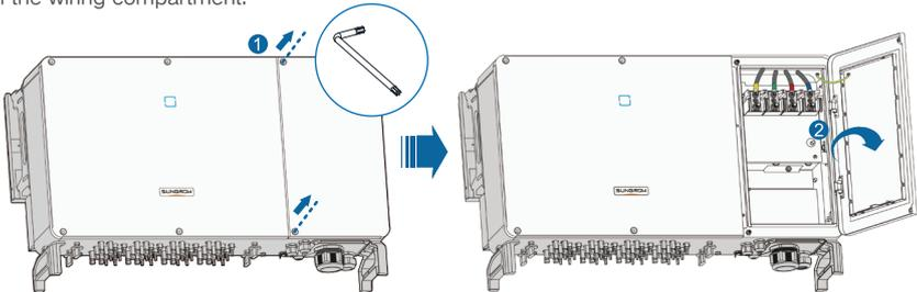
**Step 2** Keep the wiring compartment opened during wiring through the limit lever attached to the cover.
