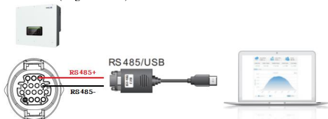
Fig.5-10 RS485 connection (cascade of monitoring between inverters)
